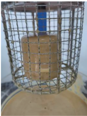
图 12 泥饼被膨润土包裹示意 Fig. 12 Mud cake wrapped in bentonite
