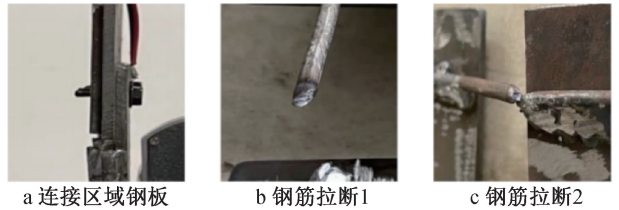
图 4 试件 S6. 3/4-J1-3 破坏现象 Fig. 4 Failure mode of specimen S6. 3/4-J1-3
