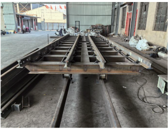
图 6 TBM 法洞内可移动式道岔 Fig. 6 Movable turnout in tunnel construction by TBM method
