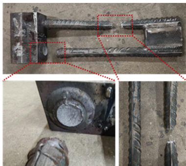
图 10 C-T 型连接件拉伸试验破坏现象 Fig. 10 Failure mechanisms of C-T type connector under tensile testing
